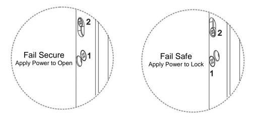
Strike is shipped from factory in fail-secure configuration. If fail-safe configuration is desired, remove screw from hole #1 as shown in above diagram and loosen screw #2. Slide screw #2 to opposite end of the slot and tighten. Install screw #1 into hole labeled fail safe.
