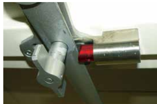
STOP SHOWN WITH SPRING LOADED PLUNGER FULLY COMPRESSED
