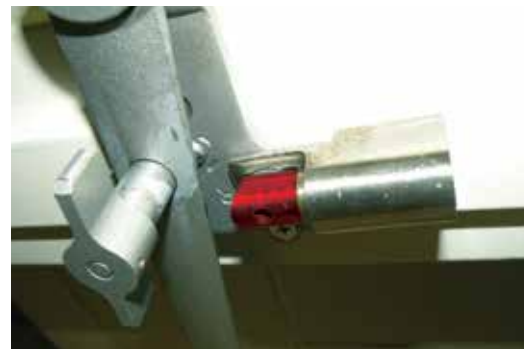
STOP SHOWN WITH SPRING LOADED PLUNGER FULLY EXTENDED
